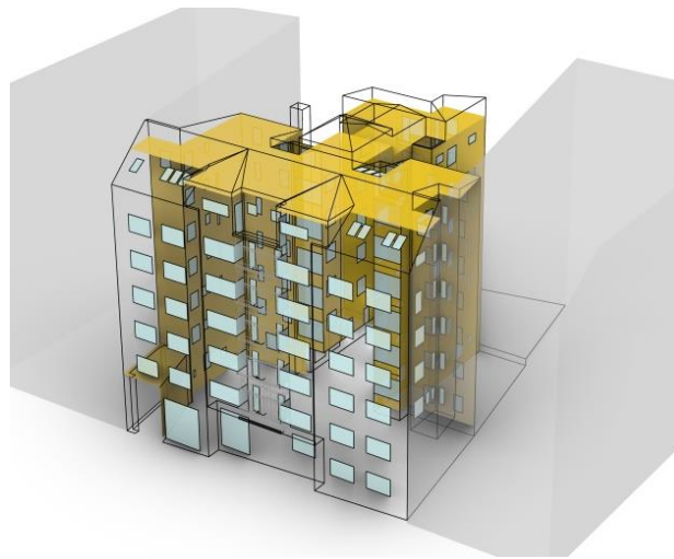
Figure 4. Illustration of the elements of the building thermal envelope upgraded in the second level of improvement
