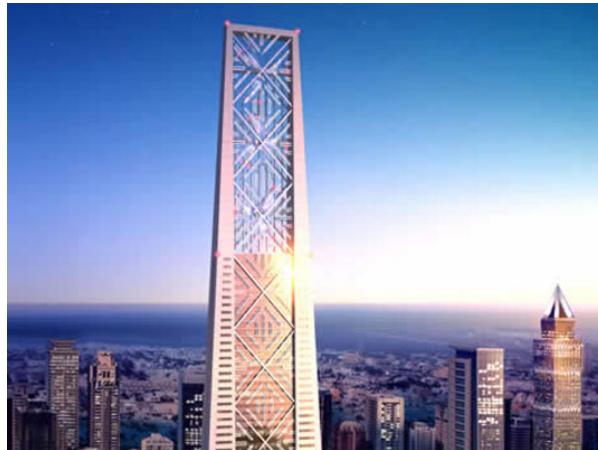
Picture1. The Tower "Lighthouse" in Dubai has 4.000 solar panels on the south side and three wind turbines, which meets its own energy needs
